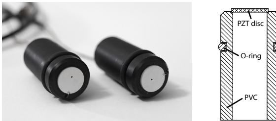
Figure 3.4: Pair of transducers made of an air-backed piezo-ceramic disc mounted onto a PVC cylinder.
