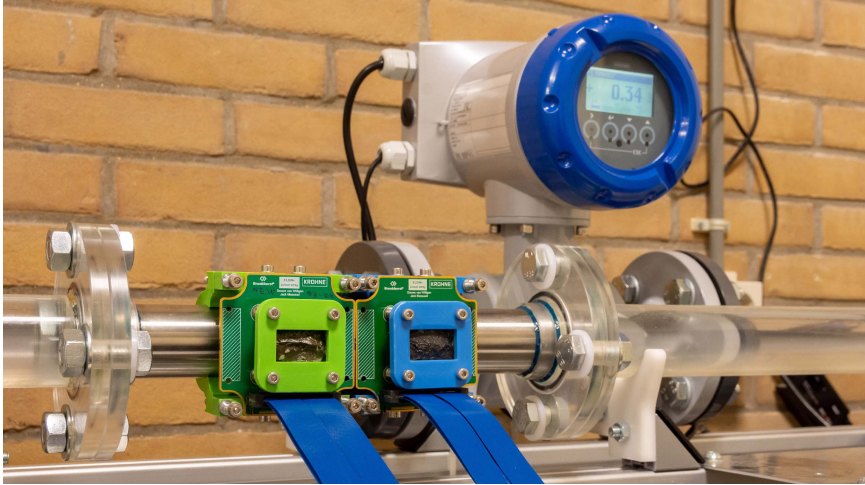
Figure 6.14: Array transducers mounted onto a steel pipe section in the flow loop, with the reference flow meter in the back.
