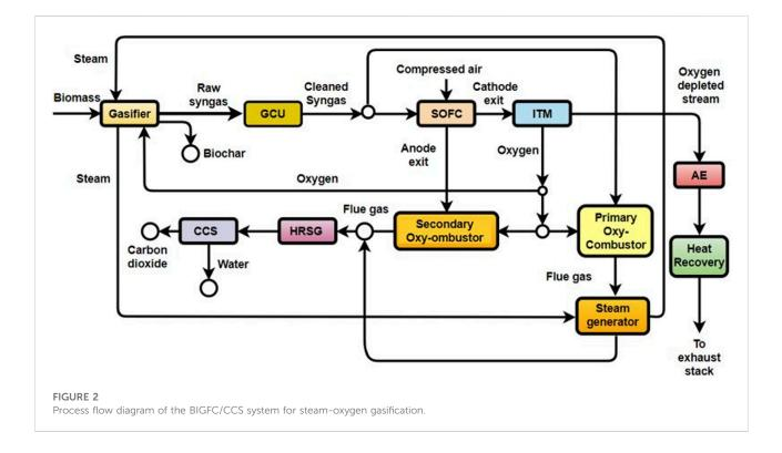
combustion chamber, and SOFC internal reforming were evaluated (Asimptote, 2014). It was also assumed that the cell resistance of the SOFC was  $5 \times 10^{-5} \Omega \text{ m}^2$  for utilizing the 85% of the incoming fuel (Thallam Thattai et al., 2017).
