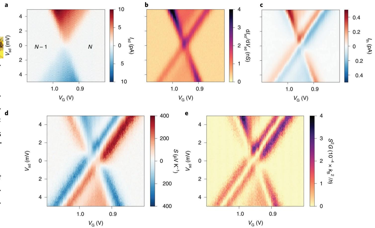
mance of a thermoelectric material is the figure of merit ZT, which takes the form ZT = $S^2GT/(K_{ph}+K_e)^6$ . Typically, a high performance device can reach  $ZT \approx 2^7$ , yet decreases drastically (ZT << 1) when it goes to low temperature. The Gd complex device has a ZT $\approx$  0.7 at T = 2 K outperforming most of the semiconductor devices.
