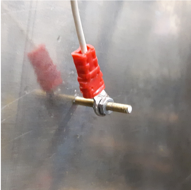
Figure 3.8: Close-up of a representative PD electrode attachment. The M2 brass bolt connects the PD wire with the specimen.
