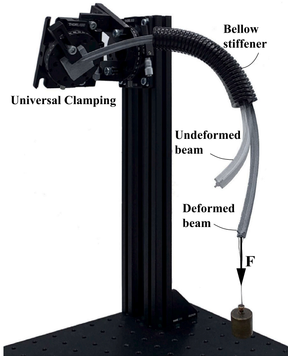
Fig. 5. The experimental setup with a suspended-weight represents the constant magnitude of the tip force and a universal joint at clamping to represent the changes in load direction. The spatial displacement of the endpoint was measured using image processing of unloaded and loaded states from two perpendicular angles.
