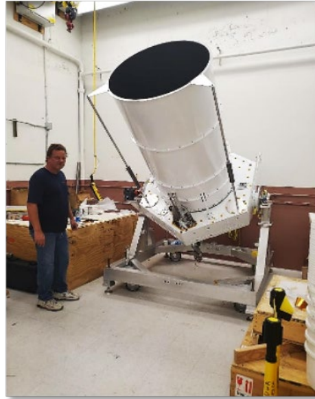
Fig. 3. GUSTO Telescope. GUSTO employs an f\#10.4 Cassegrain telescope with a 0.9m borosilicate mirror and a 14 cm aluminum secondary.
