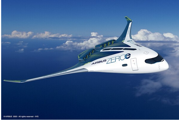
Figure 1.2: Airbus ZEROe hydrogen aircraft, blended wing concept [12]
