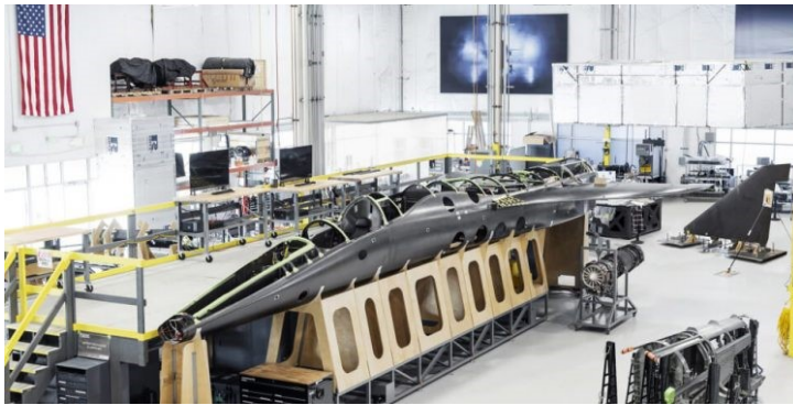
Figure 1.1: Boom supersonic's XB-1 composite + titanium fuselage [9]
