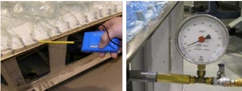
Figure 2.21: State of leakage detection technology on vacuum bags in the aircraft industry [27]
