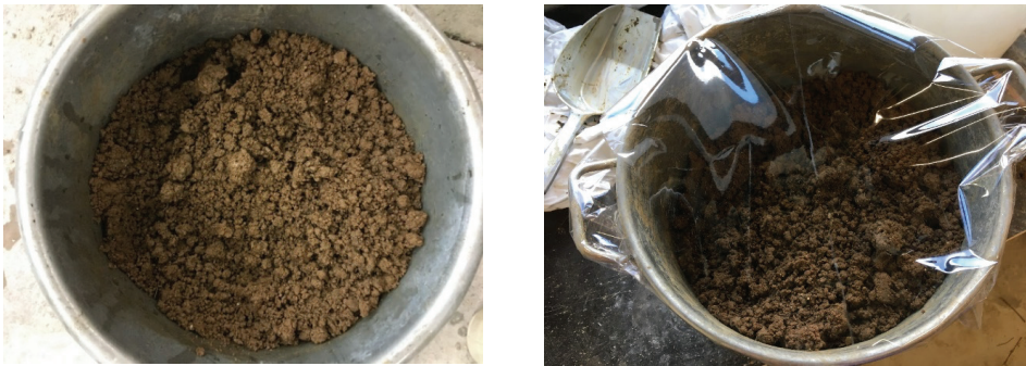
Figure 6E1: Soil cow-dung mix stored in a metal container and sealed with plastic fastened through rubber bands.
