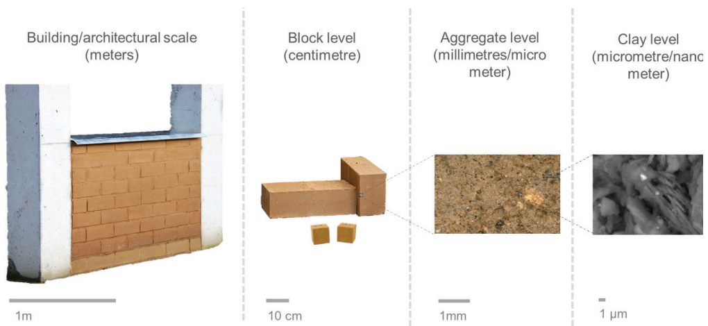
Figure 4.2: Earthen materials at different scales / levels. Left to right: An earthen wall (made from compressed earth blocks); compressed earth blocks; a microscopic image showing various aggregates and clay matrix; and a microscopic image of clay particles. Scale bars below the images provide size reference.
