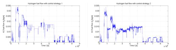
Figure 11 Hydrogen fuel flow with more energy efficient control strategy on the right
