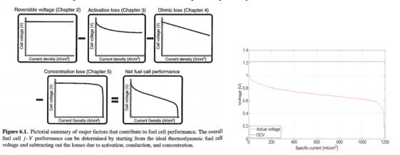
Figure 9 Build-up of FC characteristic, ref [16] (left) and FC characteristic from model (right).
