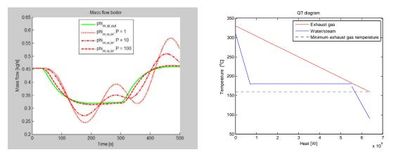
Figure 8 Feed water mass for different proportional gain settings (left) and Q-T diagram for reduced load and increased pressure (right)
