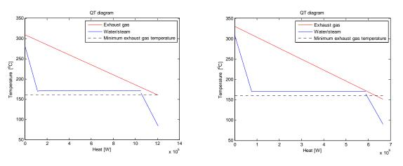
Figure 6 Q-T diagram for design condition (left) and reduced load (right). The
