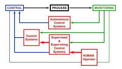
Figure 2 Control & Monitoring: layers and levels
