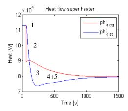
Figure 7: Heat flow in super heater after exhaust gas mass flow step
