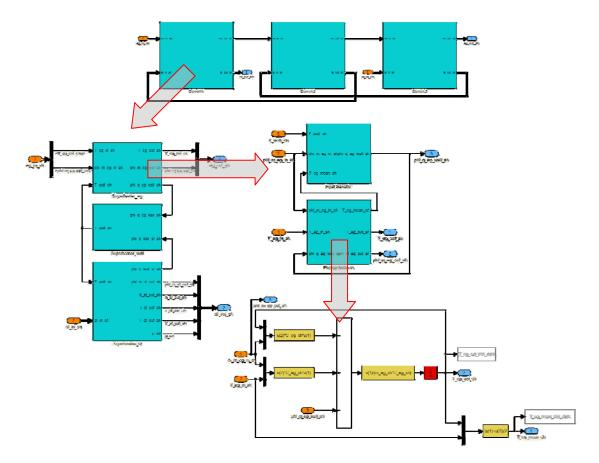
Figure 5 Example of model structure: the super heater model consist of three elements (top) each element has a exhaust gas (eg) side, a wall and a steam (st) side and a wall (middle left), the exhaust gas side comprises of a heat transfer calculation and a energy balance, the energy balance is a straightforward simple implementation of the first law of thermodynamics, resulting in the average temperature.
