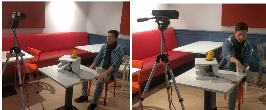
FIGURE 1 Technical setup: the participant is seated at a dining table with two bowls with identical chocolates; the robot is placed on the table at an equal distance from the bowls, performing nonverbal behaviors.
