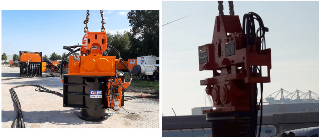
Fig. 4. The GDP shaker (left) and the Axial vibro-hammer CV-25 (right).
