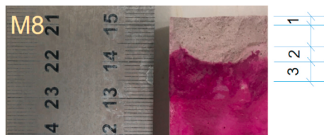
Fig. 7. The positions where powders were extracted, using slag M8 paste as an example. 1: fully carbonated area; 2: transitional area; 3: mildly carbonated area.
