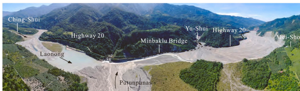
Fig. 5. Composite aerial view of the valley segment showing tributaries, Highway 20 and the along-river Minbaklu Bridge after the most recent episode of river aggradation in August 2021.
