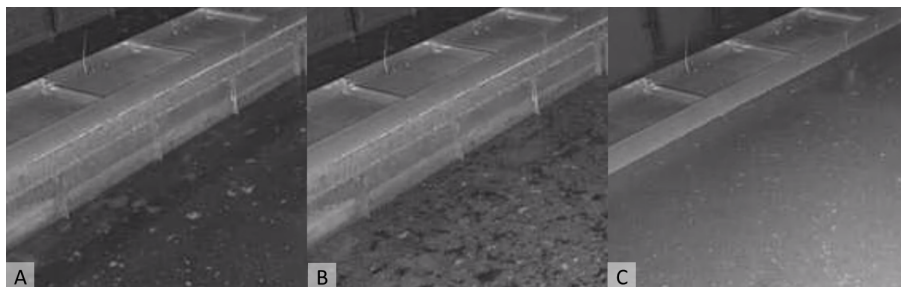
Figure 2.4: Degasification and the resulting floatation of biomass during feeding in a batch without stripping: (A) VER = 0% (B) VER = 20% (C) VER = 40%.
