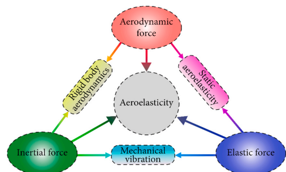
Fig. 7. Collar's triangle: interaction of different forces [66].
