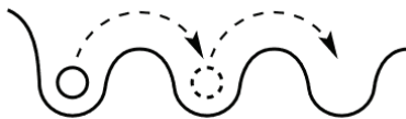
Figure 5.7: Ion hopping between sites when the thermal energy and applied AC frequency conditions are met. This process is represented by the C in the (RC) circuit. Image adapted from Ref. [25]
