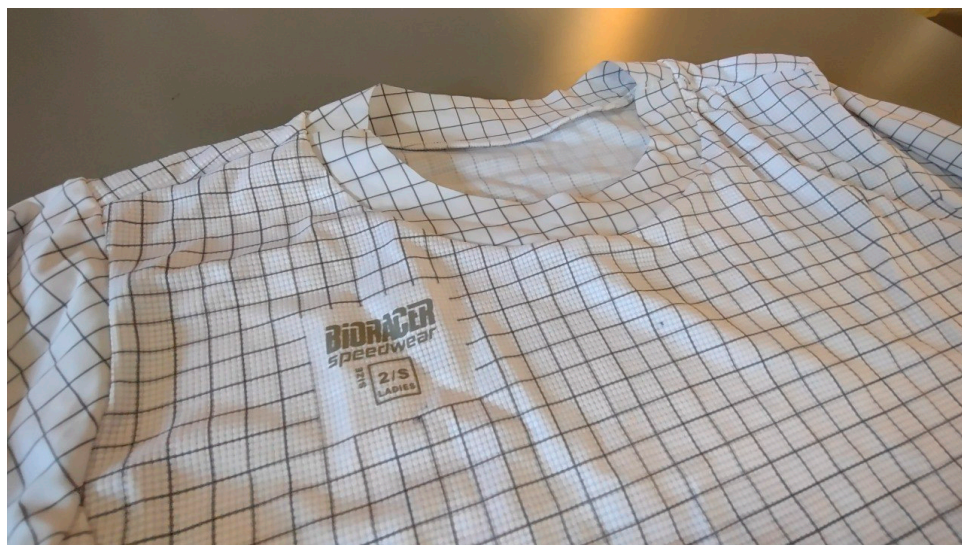
Figure 2. Custom made research garments in the standard confection sizes. The custom print consists of a 1 \times 1 cm grid of lines that aid in 3D scanning and measuring of stretch.
