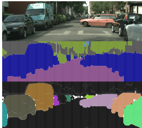
Figure 4.1: Top: Input RGB image (corresponding disparity image not shown). Middle: Semantic Stixels [1] use a semantic segmentation CNN to create a compact stixel representation which accounts for class boundaries (stixel borders: white lines, arbitrary colors per class). Note that a single stixel sometimes covers multiple instances, e.g. multiple cars. Bottom: The proposed Instance Stixels algorithm also accounts for instance boundaries using additional information learned by a CNN and clusters stixels into coherent objects (arbitrary colors per instance).
