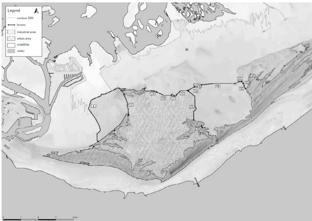
Fig. 6. Alternative 3: collective protection of population and freshwater source by adding levees to the existing landscape (20 feet contours) to create a protected zone
