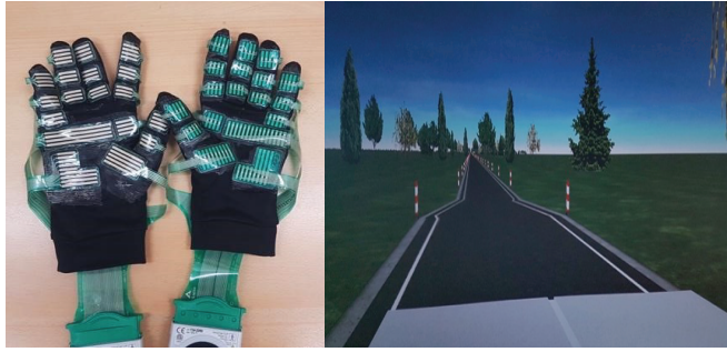
Figure 3.2. The used grip force sensors (left), and the simulator environment (right) for the 500m road narrowing including the car front.
