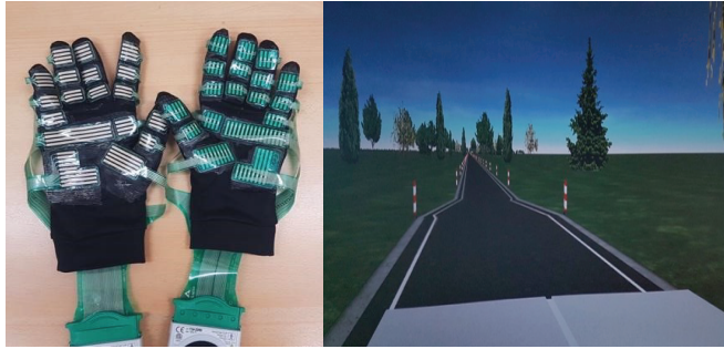
Figure 3.2. The used grip force sensors (left), and the simulator environment (right) for the 500m road narrowing including the car front.
