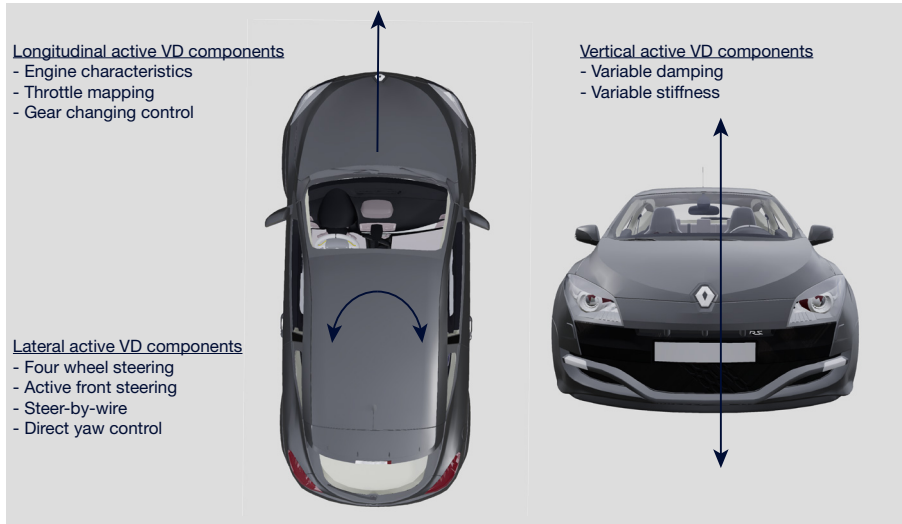
Figure 1.1. Overview of active vehicle dynamic components that can alter the vehicle dynamics.
