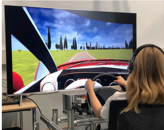
Figure 6.2. The experimental environment with a participant driving in the fixed-based simulator. The digital speedometer can be seen in light blue font, just above the bonnet.
