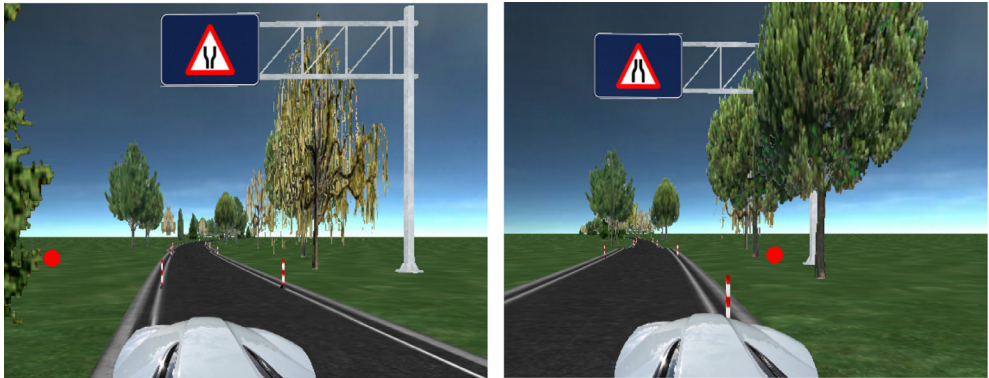
Figure 2.3. Simulator environment including the car front, transition signs and cone hit warning (i.e. red dot accompanied by a sound of 82 dB).
