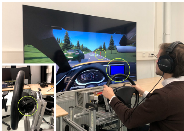
Figure 8.1. A participant driving in the driving simulator. The dashboard display shows the steering gain (SG) currently active (here colored blue, indicating low SG). The arrow next to the depicted speed indicates the advised SG level (available in the DI condition only). In this figure, participants are advised to switch ‘up’, from low SG to high SG. The left-bottom inset shows the button at the back of the steering wheel that was used to initiate SG transitions. Participants wore headphones that displayed regular driving sounds (Melman et al., 2021b).
