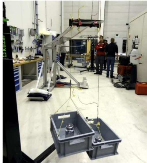
Figure 10. Static test setup—load application.
