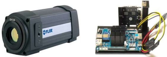
Fig. 1. FLIR SC305 infrared camera (left picture), Pine RockPro 64 (SBC) (right picture).
