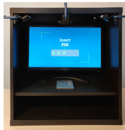
Figure 3: Our experimental setup. The cameras are visible but they can be hidden into the frame of an ATM. In all other aspects, we reproduced a common ATM layout in detail.
