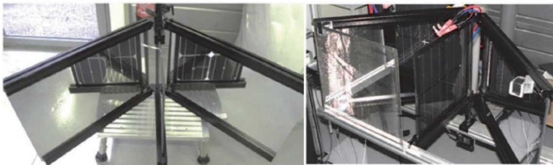
Figure 3. Two-mirror setup for bifacial PV module characterization [81].
