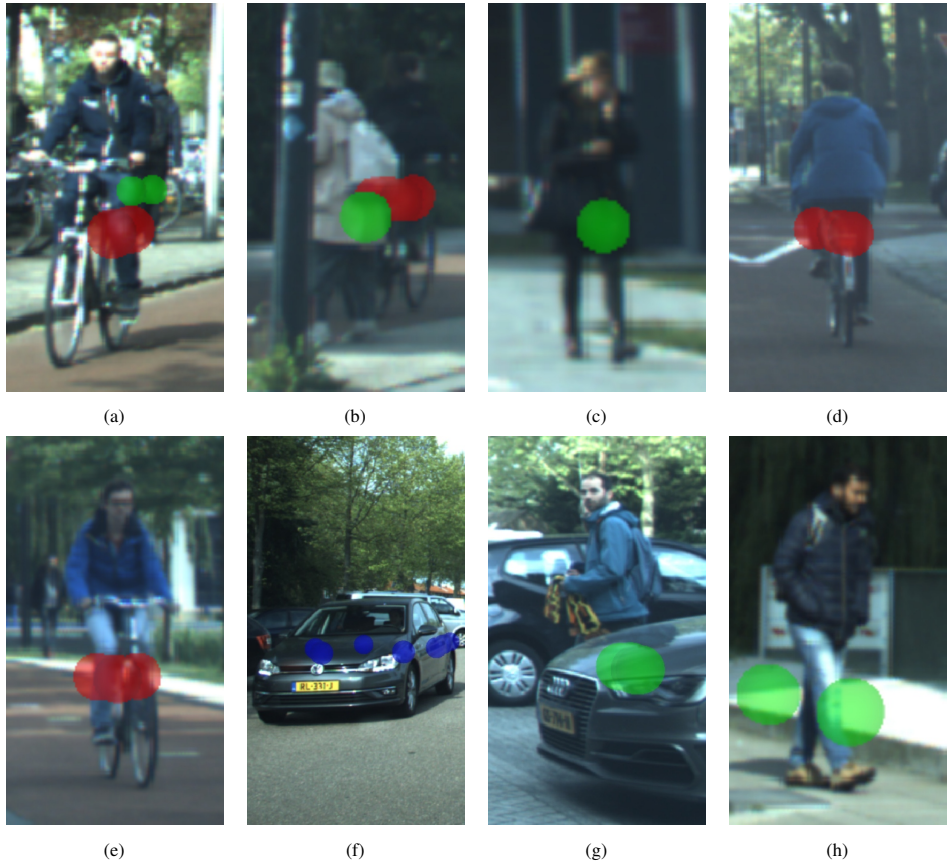
Figure 5.7: Examples of correctly classified radar targets by RTCnet , projected to image plane. Radar targets with pedestrian/cyclist/car labels are marked by green/red/blue. Static objects and the class other are not shown.
