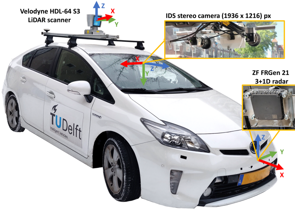
Figure 6.3: Recording platform. Our Toyota Prius 2013 platform is equipped with a stereo camera setup, a rotating 3D LiDAR sensor, a ZF FRGen 21 3+1D radar, and a combined GPS/IMU inertial navigation system.
