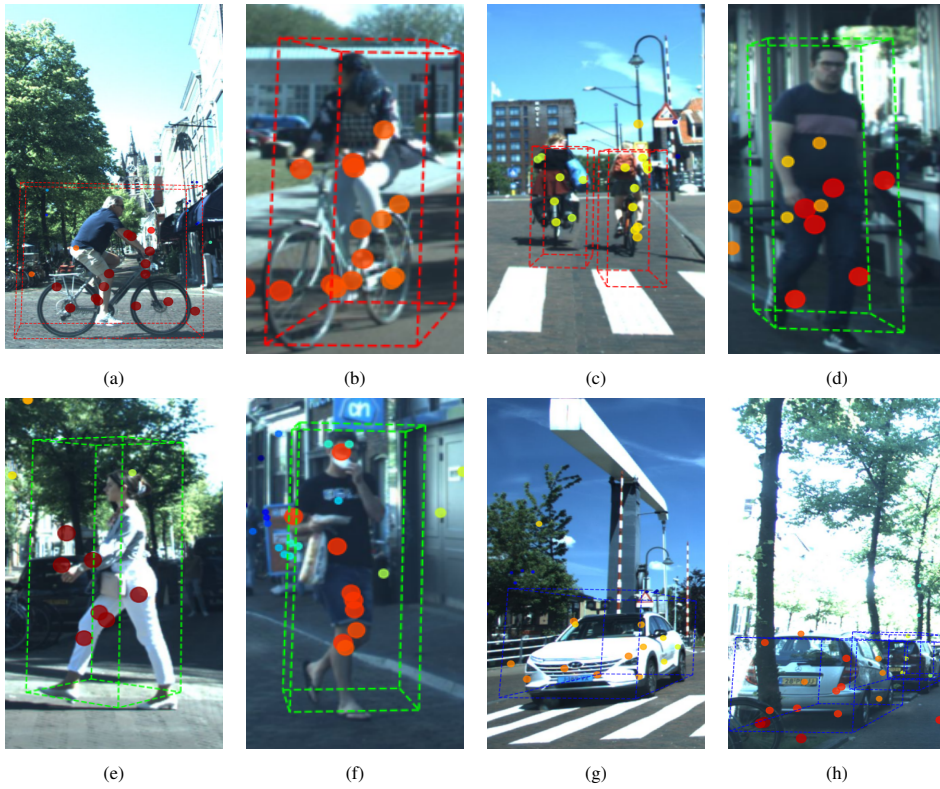
Figure 6.7: Examples of correctly detected objects by PP-radar projected to the image plane. Car/pedestrian/cyclist detections are shown as blue/green/red bounding boxes. Dots are radar targets colored by distance from the sensor.
