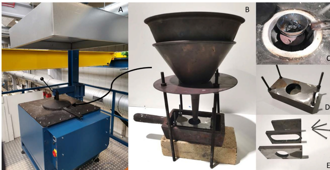
Figure 3. Melting Oven. A: The induction furnace for melting of the Zamak laryngoscope blades. B: All-in-one casting setup placed in the melting oven. C: Top bowl with filter allows only the Zamak to pass. D: Cast with riser. E: Exploded view cast with riser.
