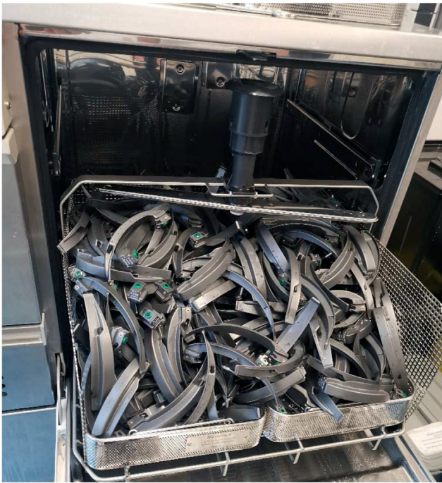
Figure 2. Thermal disinfection with customized insert rack for disinfection of blades in larger quantities.
