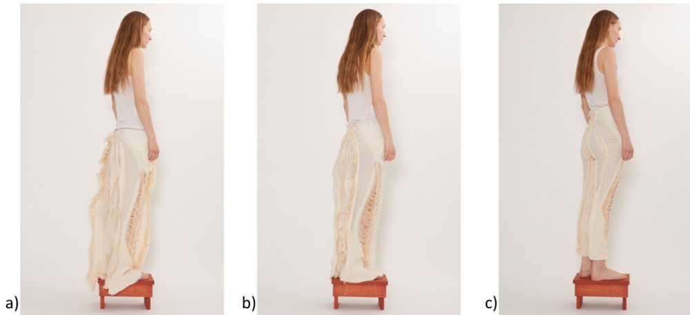
Figure 19. a) Woven textile-form unshrunk. b) Woven textile-form shrunk on the mould so that the garment fits to the waist of model. c) Woven textile-form shrunk in a dryer. In this case, uniform heat is applied to the whole textile but the weave structures cause large variation in the expression of the heat reactive yarn. Photograph: Amanda Johansson. Source: ©2021 Holly McQuillan, Kathryn Walters and Karin Peterson. (CC BY-NC-ND 4.0).
