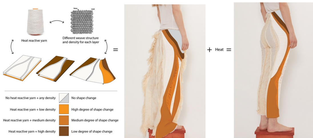
Figure 18. Yarn, weave structure and textile-form construction work in symbiosis to produce specific shape change behaviours. Source: ©2021 Holly McQuillan (CC BY-NC-ND 4.0).
