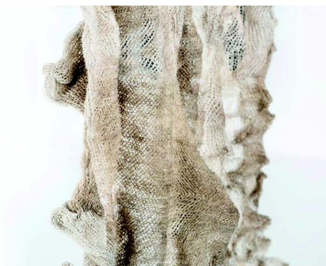
Figure 7. Knitted structure shrunk in response to cold water spray (Scott, 2018). Source: © 2018 Jane Scott (CC BY-NC-SA 4.0)
