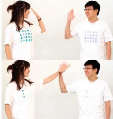
Figure 1. T-shirts display a message via thermochromic ink (Kan et al., 2015). Source: © 2012 Tangible Media Group / MIT Media Lab (CC BY-NC-ND 3.0)
