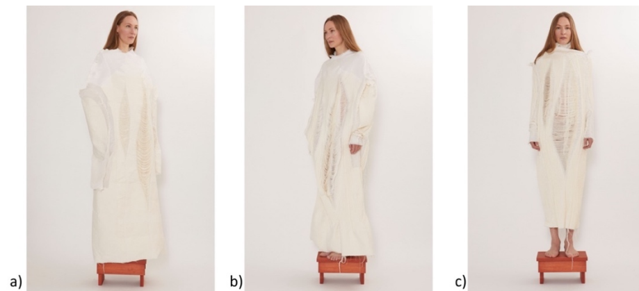
Figure 16. The woven textile-form in its many states: a) unshrunk; b) shrunk on mould using targeted heat application; c) uniformly shrunk in the dryer. Photograph: Amanda Johansson. Source: ©2010 Holly McQuillan, Kathryn Walters and Karin Peterson (CC BY-NC-ND 4.0)
