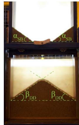
Figure 3.5 Shear angle and angle of repose in the drawdown test
