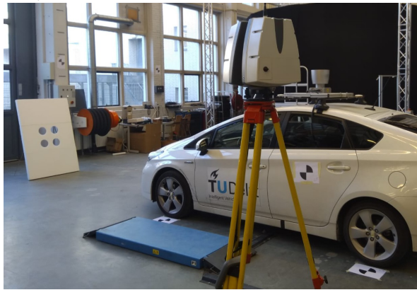
(b) Absolute calibration setup for a vehicle.
