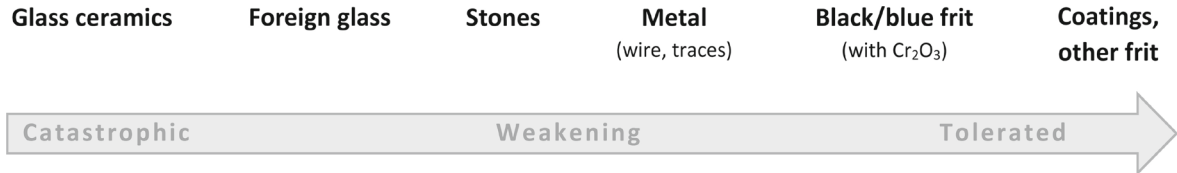
Fig. 23 Ranking of the impact each type of flaw may have on the hosting glass network
