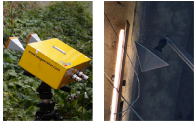
Figure 16. Radar measurement equipment. Left: radar, and right: the reflector (target).
