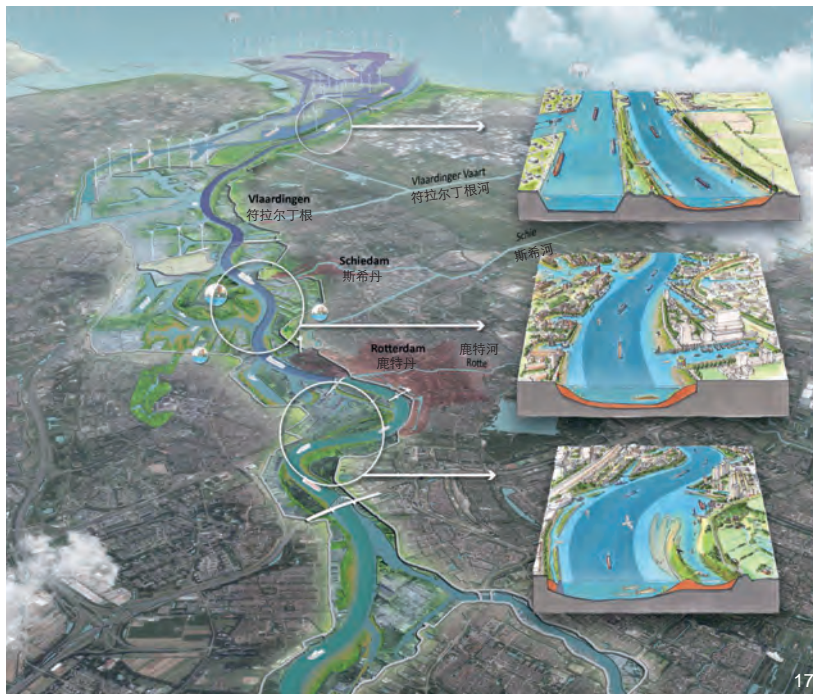
17 鹿特丹地区东侧包括新马斯河和新沃特伟赫河鸟瞰示意图。探索河床变浅变宽可能性的研究型示意图 Bird's-eye sketch of Rotterdam region with Nieuwe Maas and Nieuwe Waterweg. Study-scetch to explore the possibility of shallowing and broadening the riverbed
