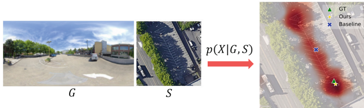
Fig. 1. Example of visual cross-view metric localization. Given a ground-level image G (left), and a satellite patch S (middle) with its local area, we aim to identify the location X within S where G was taken. Our method estimates a dense probability distribution over the satellite image. The resulting (log) probability heat map is overlaid in red on top of the satellite patch (right). Compared to the regression-based baseline that tends to roughly regress to the midpoint among multiple modes, our method captures the underlying multi-modal distribution. Our final predicted location, \operatorname{argmax}(p(X|G, S)) , is closer to the ground truth. (Color figure online)
