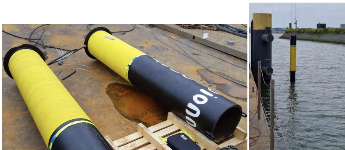
Figure 1 Left: two mantels of which only the right one is used. Right: picture of a mantle being installed on a pole.
