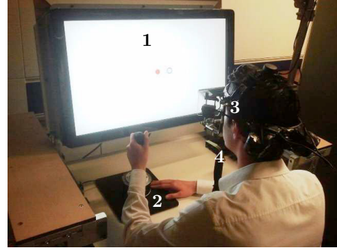
Fig. 3. A participant seated in the measurement setup consisting of a screen (1), a joystick (2), an infrared eye tracking system (3), and a chin rest (4).
