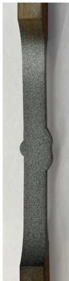
Fig. 8. Measured surface of the unmilled welded coupon specimen.
