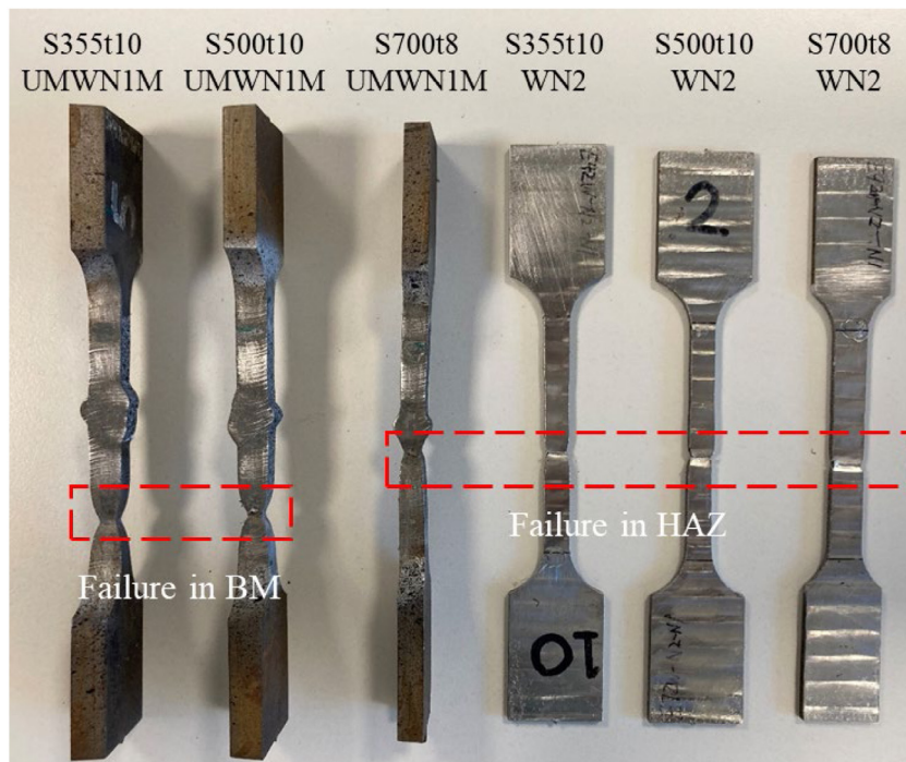
Fig. 16. Failure of milled and unrolled welded coupon specimens.
