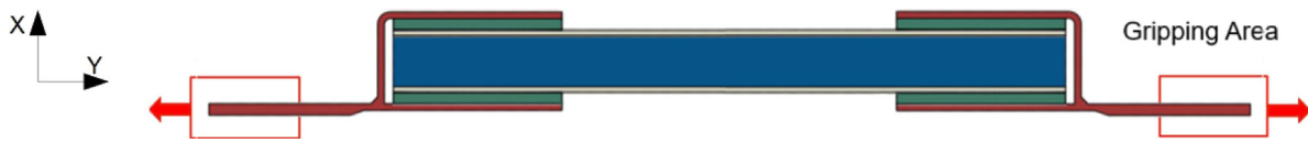
Fig. 4. The FE model for tensile tests. The loading is applied in the gripping region.
