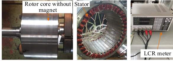
Fig. 18. Prototypes manufactured and the LCR meter. (a) Serial connection (b) Parallel connection.
