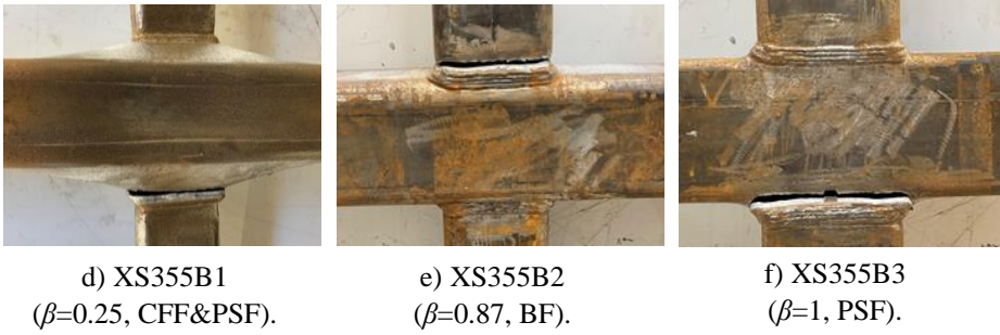
Fig. 6.7 Failure modes of S355 X-joints.
