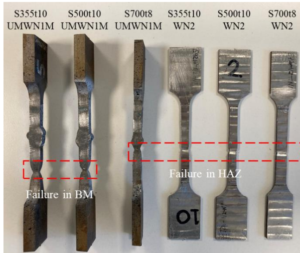
Fig. 4.11 Failure of milled and unmilled welded coupon specimens.
