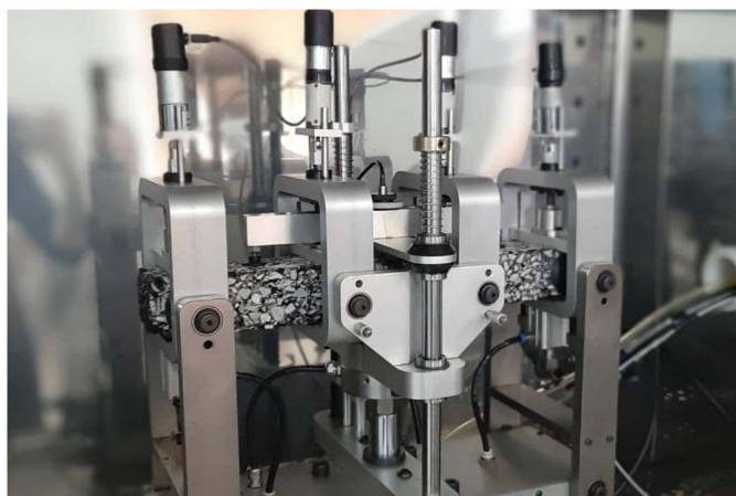
Fig. 7. The beam fatigue test setup.
