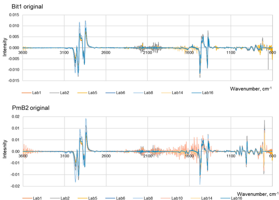
Figure 4. 1st derivatives of IR spectra of Bit1 and PmB2 from different laboratories.
