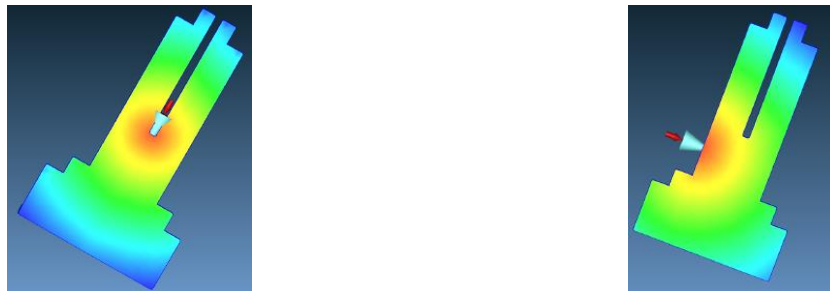
a) Gate location optimisation by software b) Adapted gate location by students
