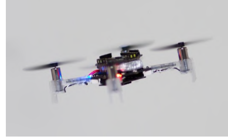
Fig. 9. Crazyflie, a 39-gram MAV from company Bitcraze.
