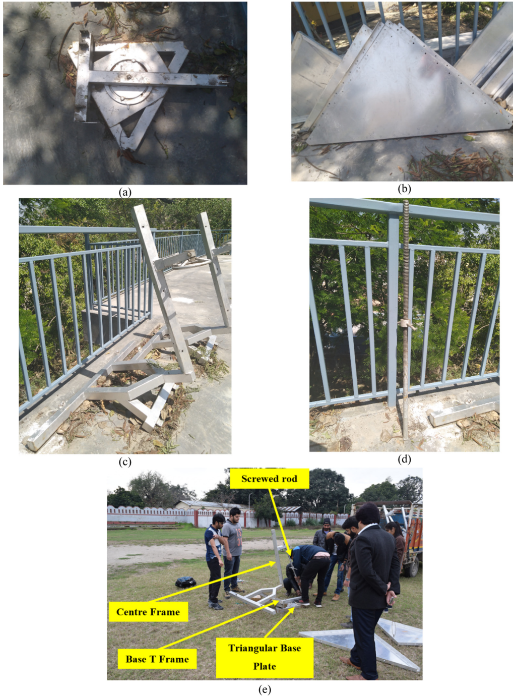
Fig. 6. Parts of the corner reflector (a) base T frame of the Triangular Trihedral corner reflector (b) triangular reflecting panels (c) Center Frame (d) Screwed rod (e) Deployment of the Triangular Trihedral corner reflector.
