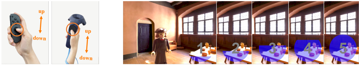
Fig. 4: Resulting prototypes. Two annotation input techniques (left): Joy-Con joystick controller (up/down), touchpad (up/down). DotMorph (right): a circle with tick label fixed to the bottom-right corner of the viewport, which varies in Fill (up/down) with annotation state.
