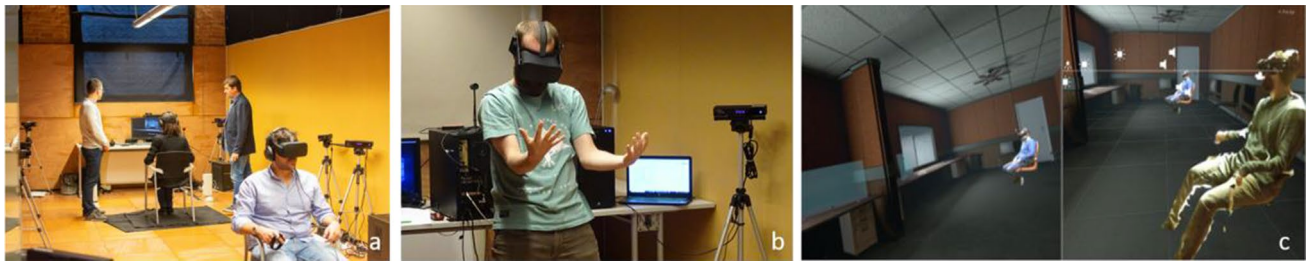
Fig. 1 Users Experiencing our SocialVR platform: a The lab and system setup; b A user recognizing his hands (self-representation in VR); c Two users integrated in a Social VR scenario
