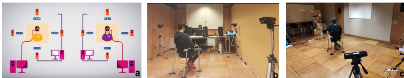
Fig. 8 Experiment Setup: a illustration of the apparatus; b and c general views of the lab and experiment rooms, with the capturing setups and users in the center of the capturing area
