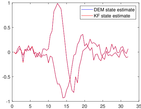
Fig 3.6: State estimation of KF and DEM coincides when noises are white and inputs are not modelled. Here \Pi_x is assumed to be e^0 I_{2 \times 2} during estimation. \sigma = 10^{-9} and dt = 0.5s .
