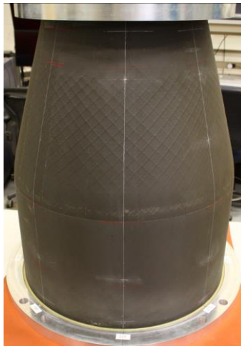
Figure 5. Test article potted in the end rings.
