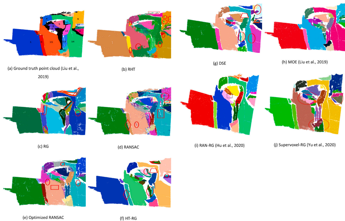
Fig. 12. Comparison of segmentation results for different methods vs. ground truth data for PC1; Raw dataset provided by Lato et al. (2013) and visualization of methods presented by Liu et al. (2019).
